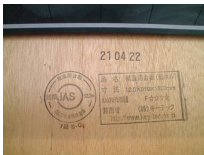
JAS Class 1 Structural Plywood 12mm
