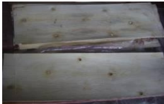
Figure 68. Knot defects in veneer of pulai wood.
