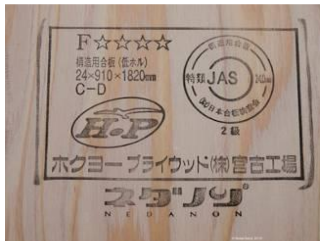
JAS Structural Plywood 24mm
