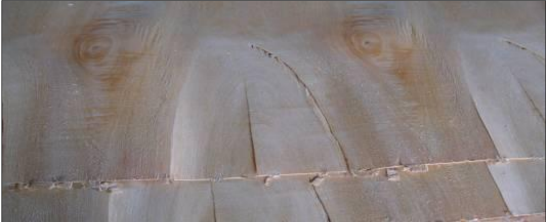
Figure 59. The quality of veneer produced from SDL
