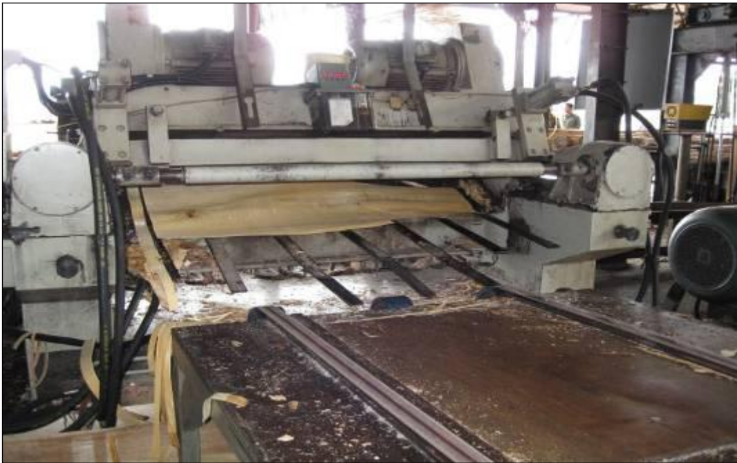
Figure 58. Veneer production using SDL as raw material
