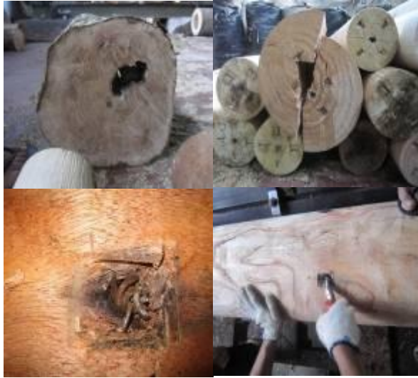
Figure 67. Physical condition of small diameter wood stems which were used as raw materials of LVL
