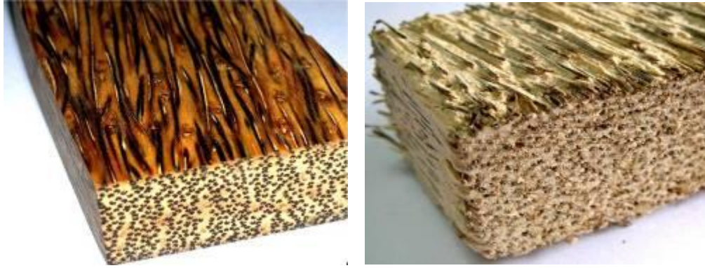
Fig. 31: Treated (left) and untreated (right) oil palm wood
