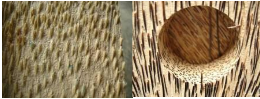
Fig. 29: Oil palm wood showing bad planing and boring properties
