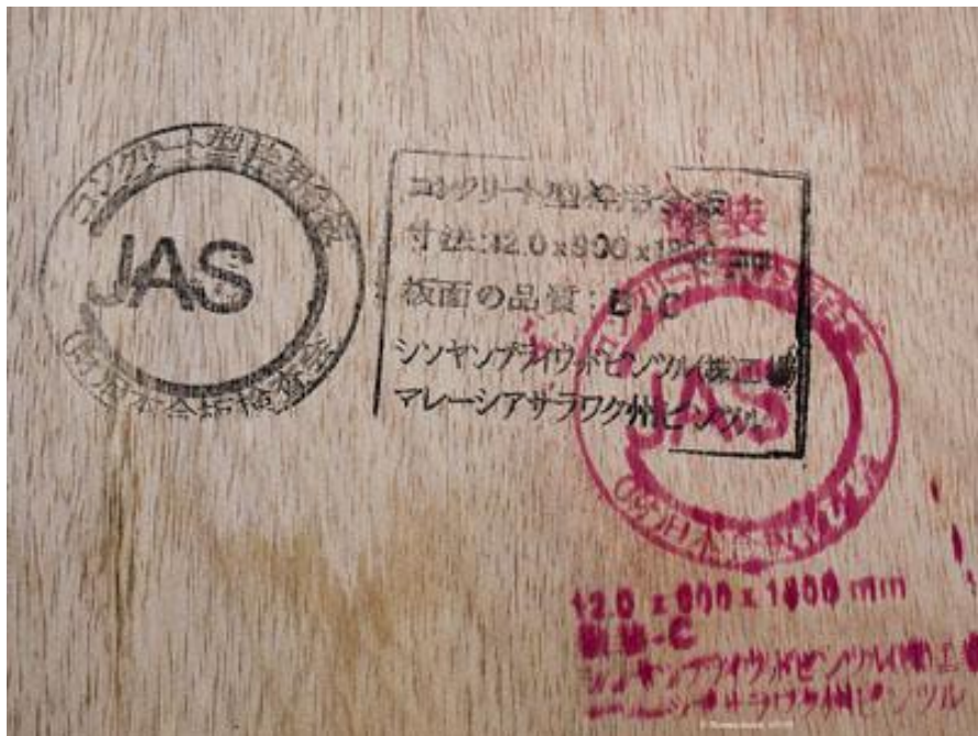
JAS Coated Concrete Form Plywood 12 mm
