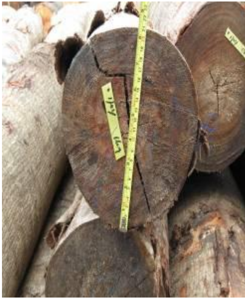
Figure 56. SDL check and split defects and how to minimize them.
