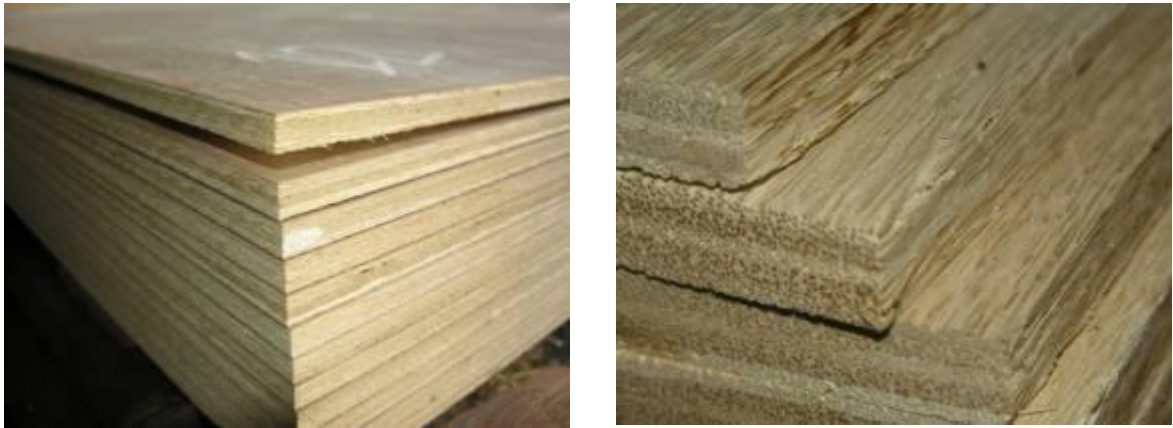
Fig. 30: Oil palm veneers are used for plywood (left) and LVL (right) productions
