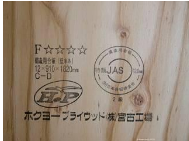
JAS Structural Plywood 12mm
